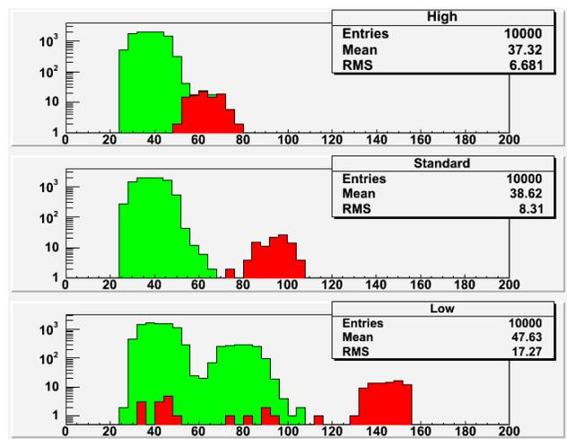
Figure 5. Latencies (msec) through the U/B module in three performance levels; initial packets in red, others in green.
