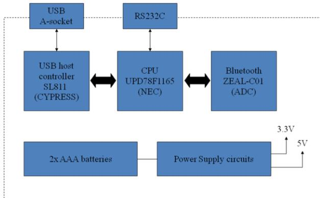
Figure 3. Block diagram of the prototype U/B module.
