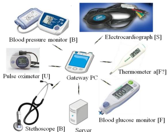
Figure 1. A versatile nurse support system using Bluetooth [B], FeliCa [F], and USB [U] & RS232C [S] over U/B module.
